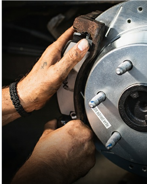
Image 3.1: A close-up view of a hand installing a new brake pad into a caliper assembly, demonstrating a step in the brake pad replacement process.
