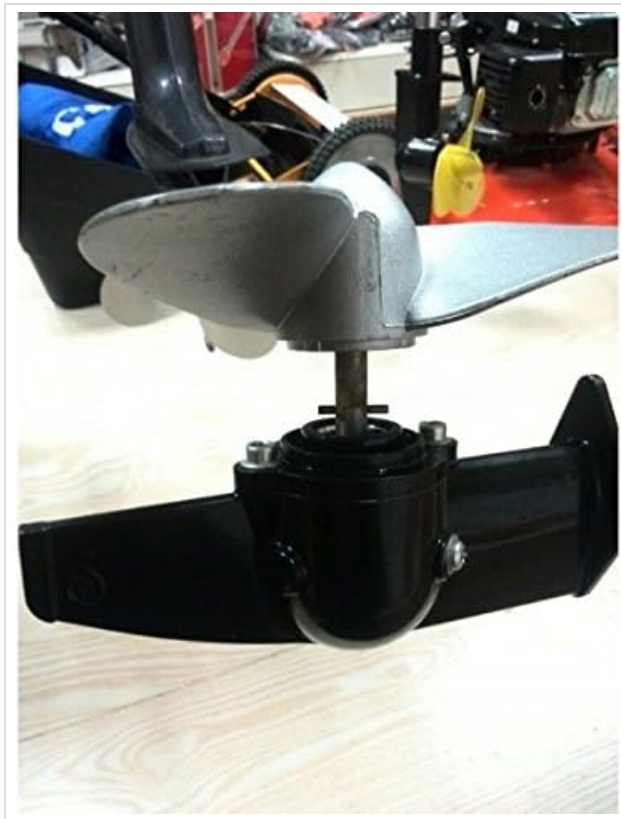
Image: The propeller and lower unit of the AQUAPARX outboard motor.
