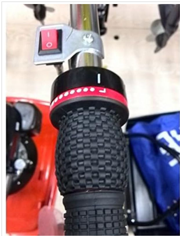
Image: Close-up view of the throttle grip on the tiller handle, showing speed markings.
