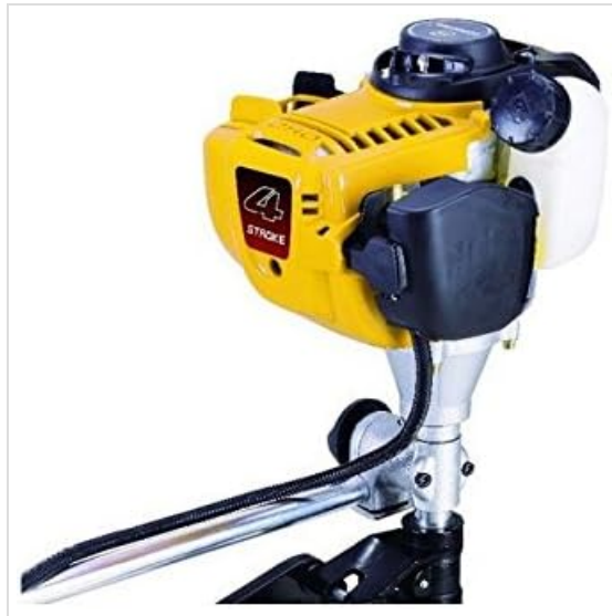
Image: The engine head of the AQUAPARX 4T - 1.3 HP Outboard Motor, showing the '4 STROKE' label.
