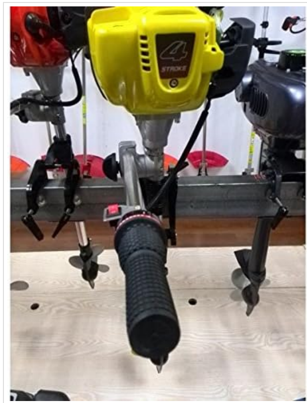
Image: Close-up view of the red kill switch button located on the tiller handle.
