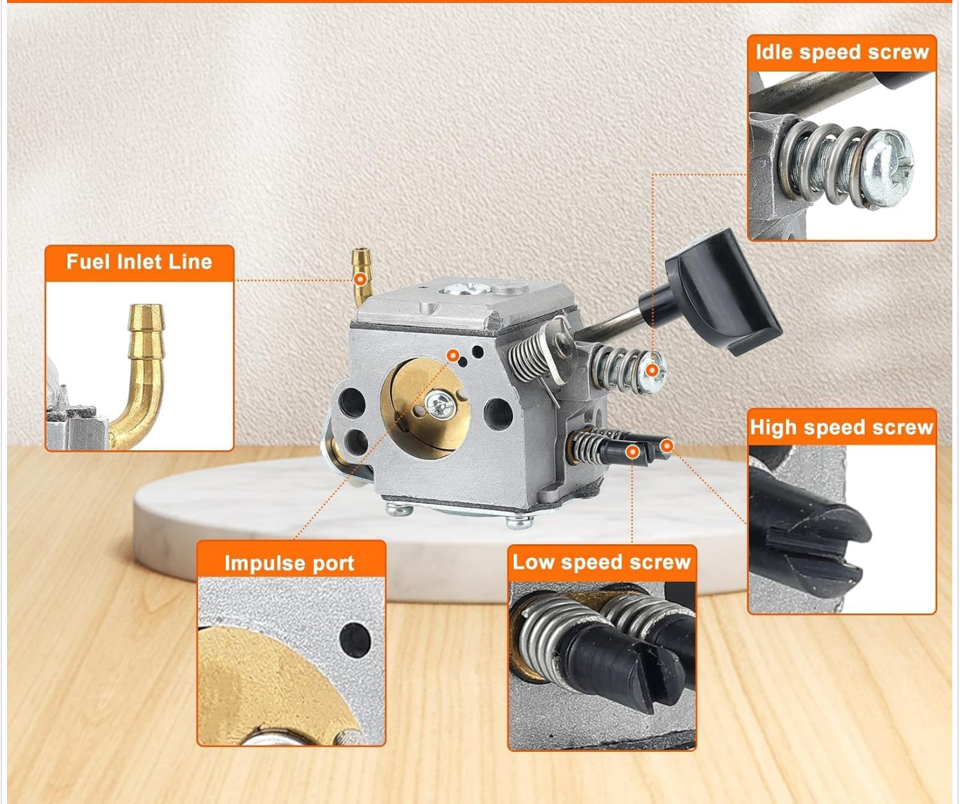
Figure 5: Tunable air-fuel ratio components for efficient operation.
