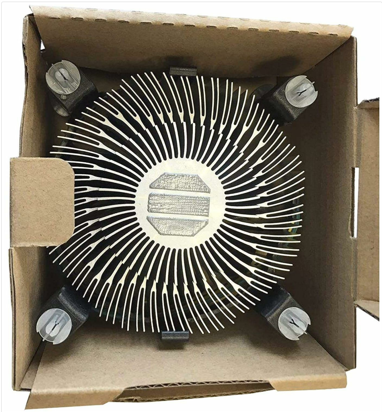
Image: Bottom view of the Intel E97379-003 CPU Cooler, highlighting the aluminum heatsink fins and the four plastic push-pin mounting mechanisms.
