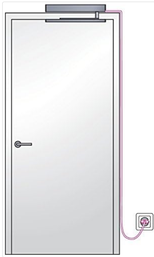
Figure 2: Diagram illustrating the power connection for the Doortronic system.
