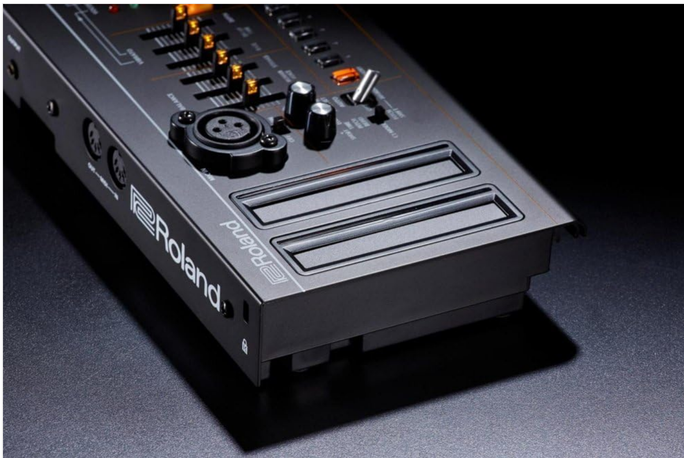
Figure 3.2: Ribbon controllers for expressive control.
