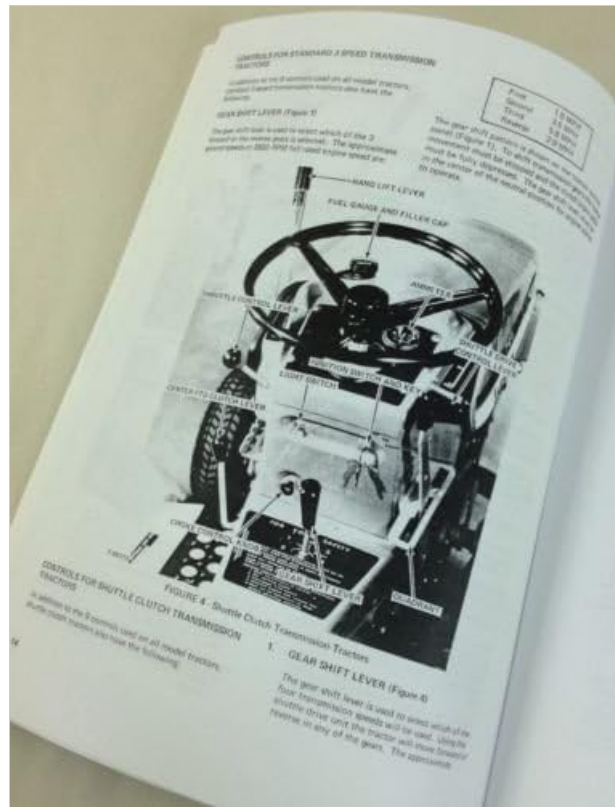
Figure 2: Detailed view of the dashboard controls, including the gear shift lever, ignition switch with key, fuel gauge, and light switch. This image helps identify specific controls for starting and operating the tractor's various functions.
