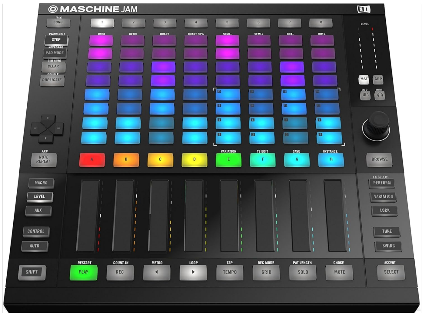
Figure 1: Top-down view of the MASCHINE JAM controller, showing the 8x8 pad matrix, Smart Strips, and various control buttons.
