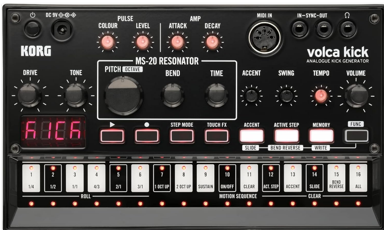
Figure 1: Front view of the Korg Volca Kick, showcasing its controls and 16-step sequencer.
