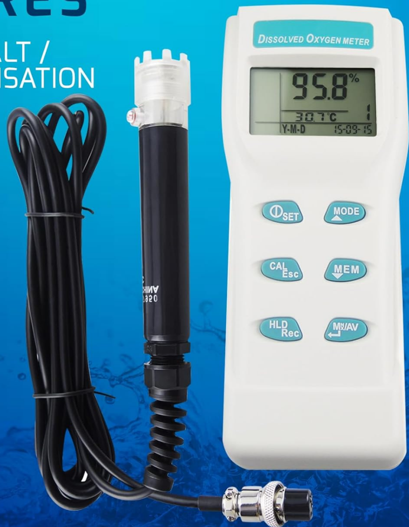
Image 5.1: Operating features of the Dissolved Oxygen Meter.
