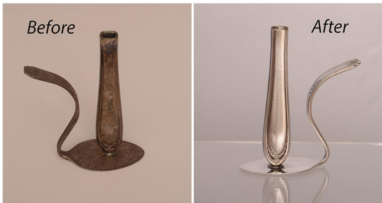
Image 3.3: Before and after polishing results on a tarnished silver item.
