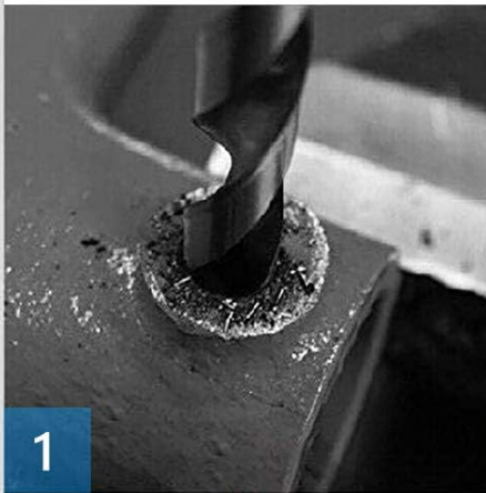
1 Drill Out The Damaged Thread Using The Correctly Size Twist Drill Bit Provided
