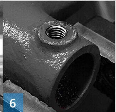
6 Thread Is Repaired And Ready To Use
