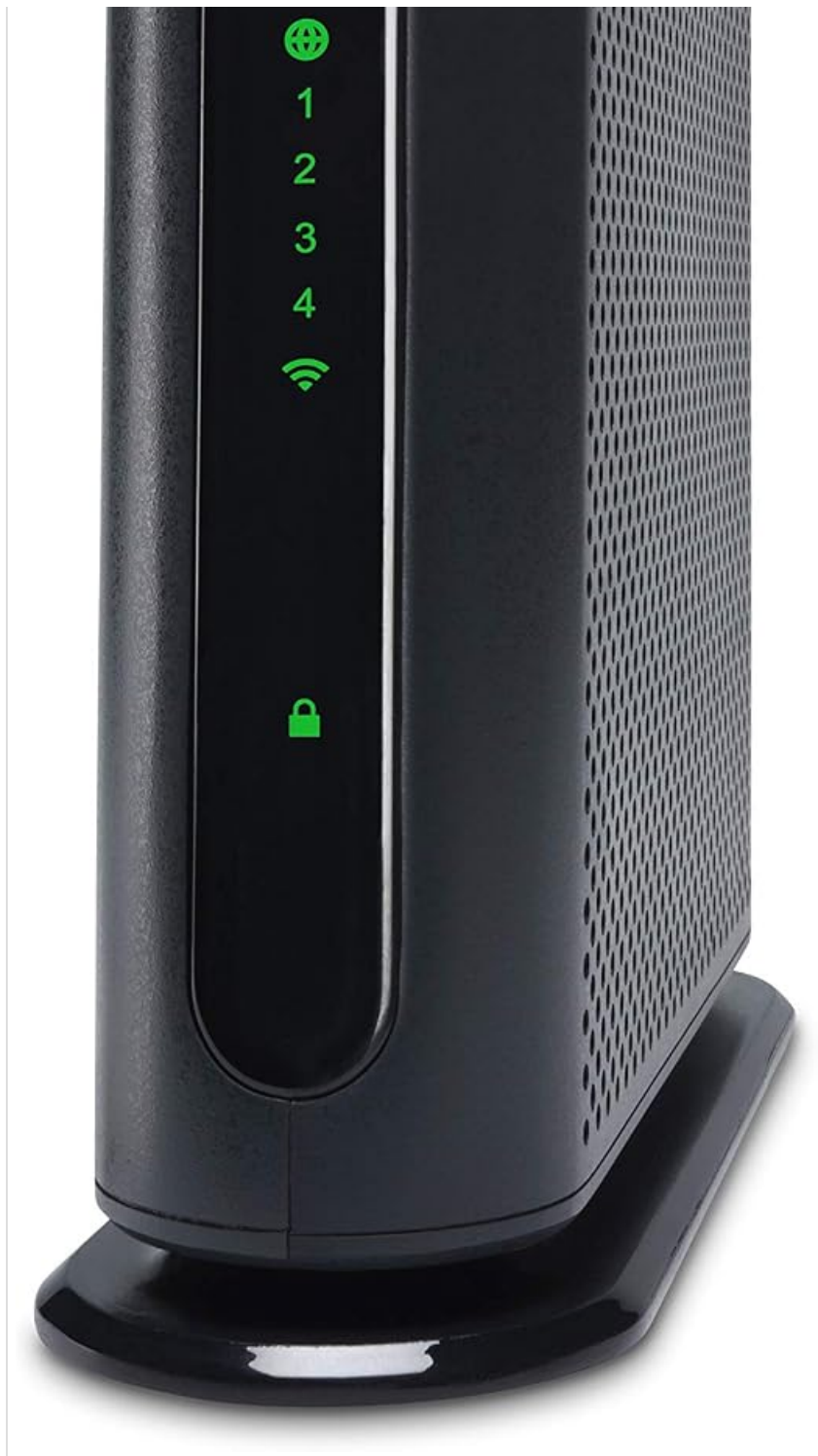
Image: Front view of the Motorola MG7315, displaying LED indicators for power, upstream/downstream activity, internet connection, Ethernet ports 1-4, Wi-Fi status, and WPS/security.
