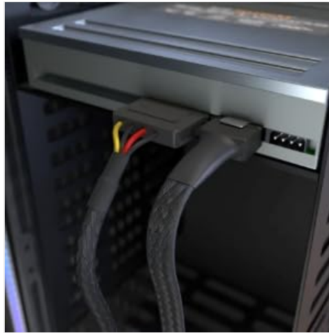
Image 3.1: A KabelDirekt SATA data cable connected to a storage drive. Ensure the L-shaped connector aligns correctly.
