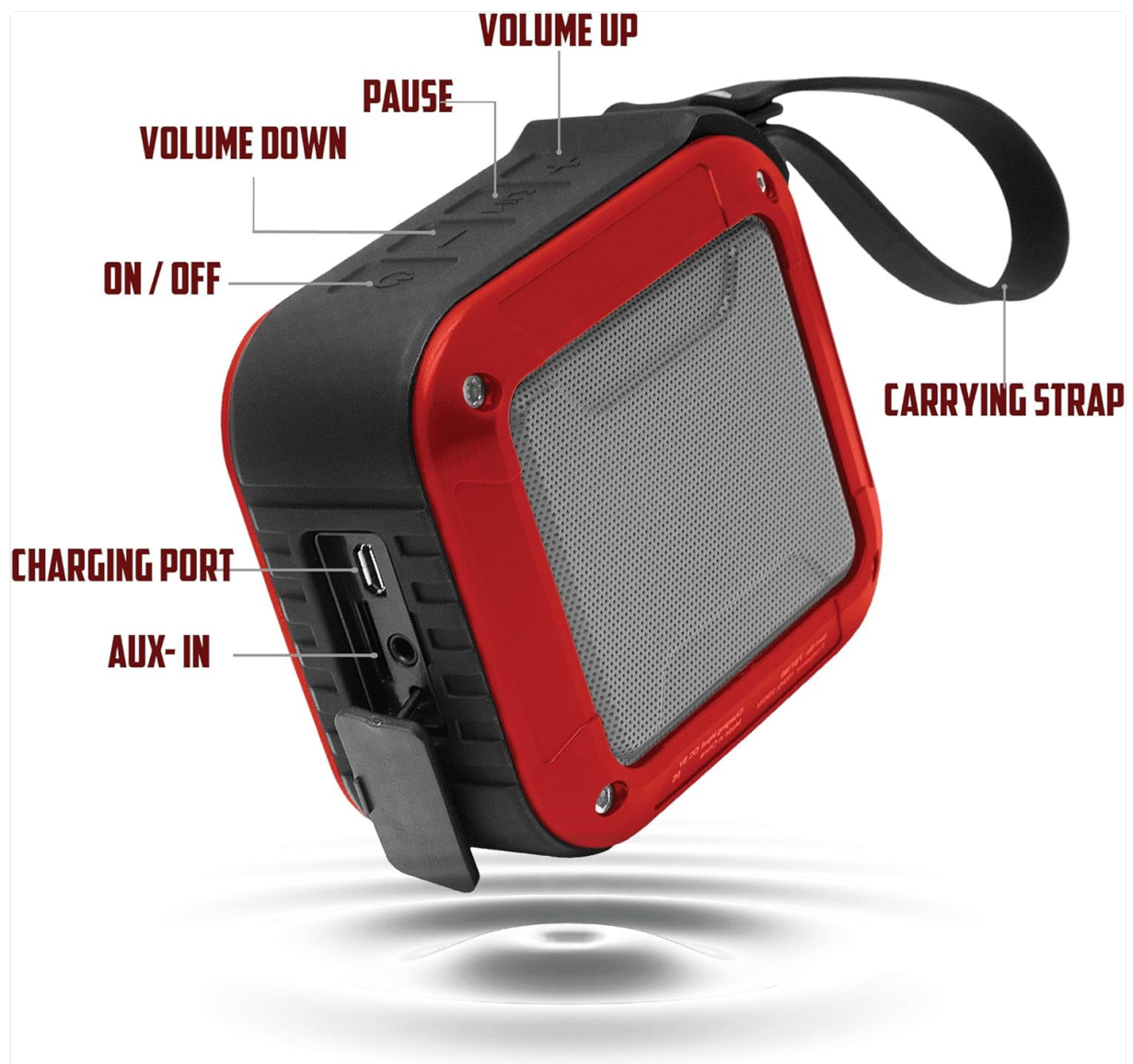
Image 3.1: Diagram illustrating the location of controls and ports on the Fisher FBT180R speaker.
