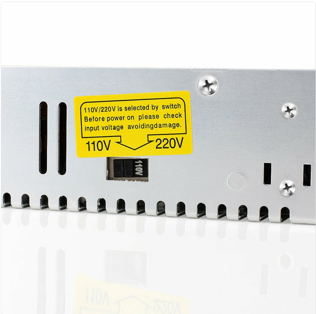
Figure 4: Close-up of the 110V/220V selector switch. Ensure this switch is correctly positioned for your region's voltage before applying power.
