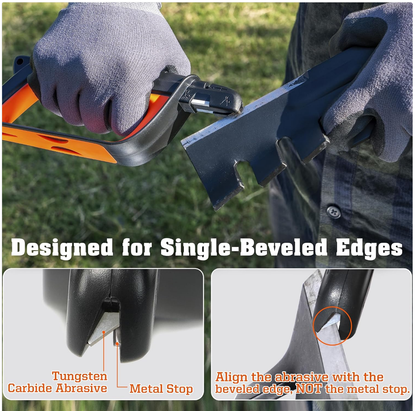
Figure 5: Illustrates the correct alignment for sharpening single-beveled edges like those on mower blades, emphasizing alignment with the abrasive, not the metal stop.
