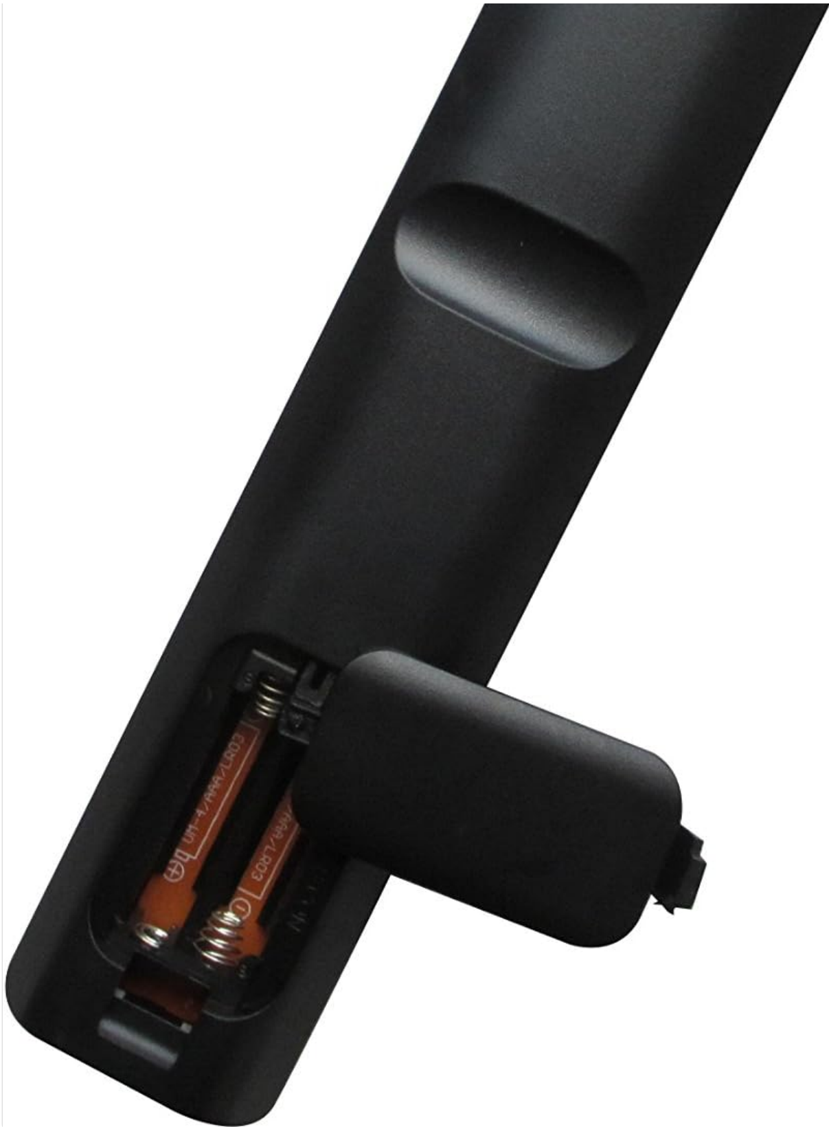
Image: Back view of the HCDZ remote control with the battery compartment open, showing two AAA batteries correctly inserted. The positive and negative terminals are visible.
