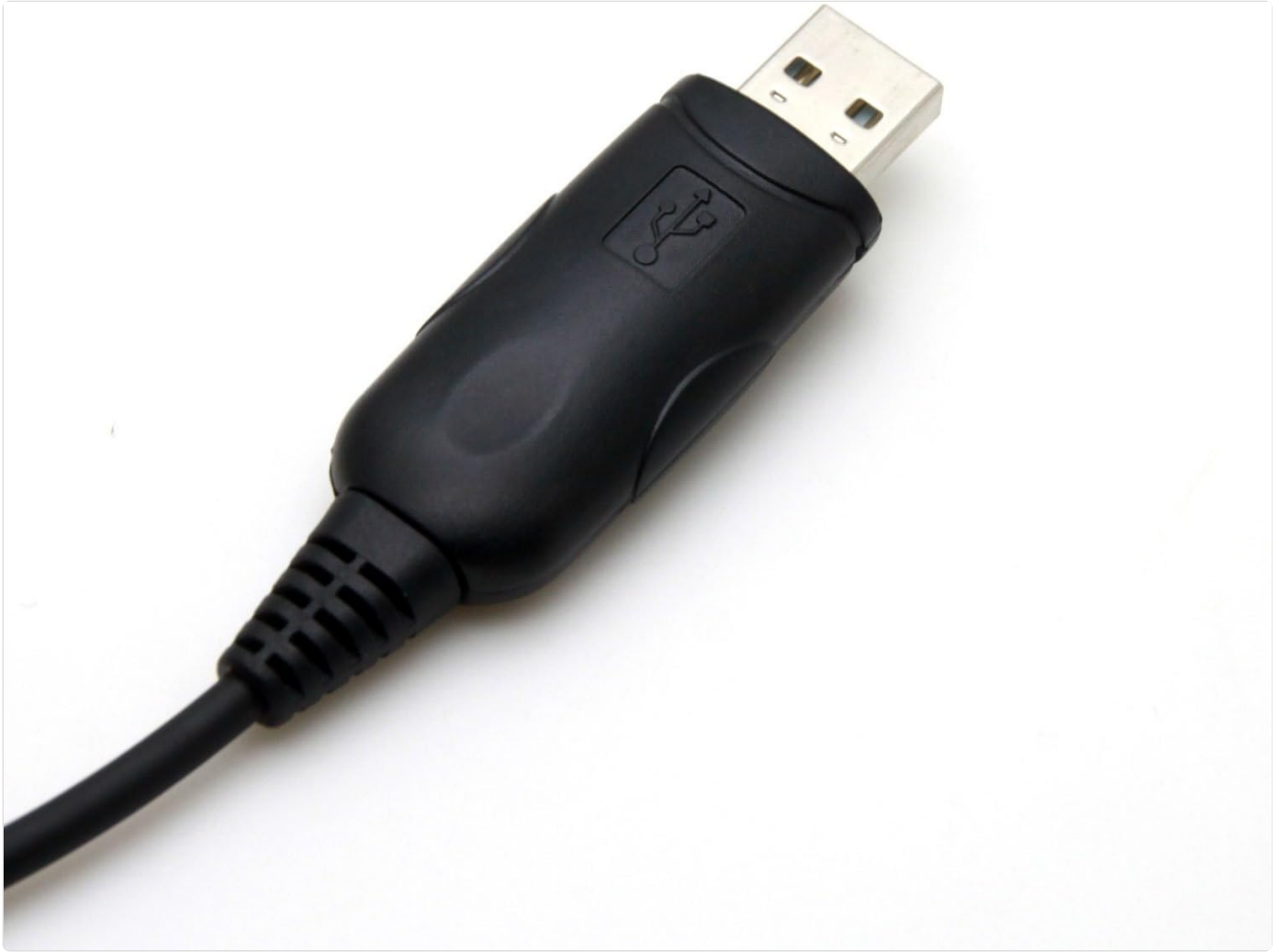
Image: A close-up view of the USB Type A connector and the inline converter module of the Kymate programming cable.
