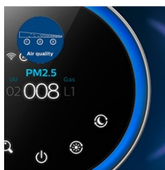
Figure 5.2: Visual representation of the air quality indicator on the control panel.
