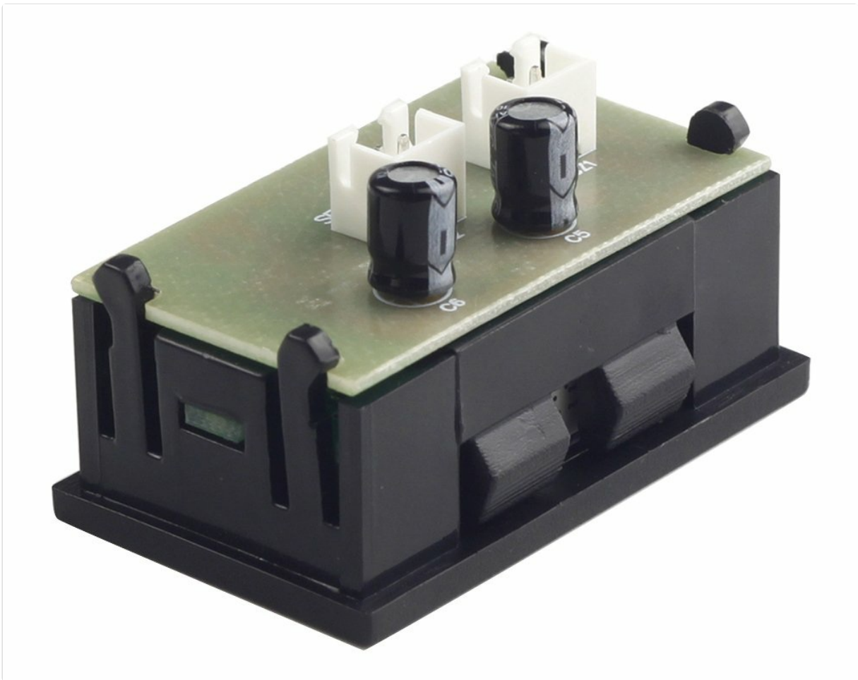
Figure 4.6: An angled rear view of the temperature meter, providing a clearer look at the power input and sensor input terminals on the circuit board.
