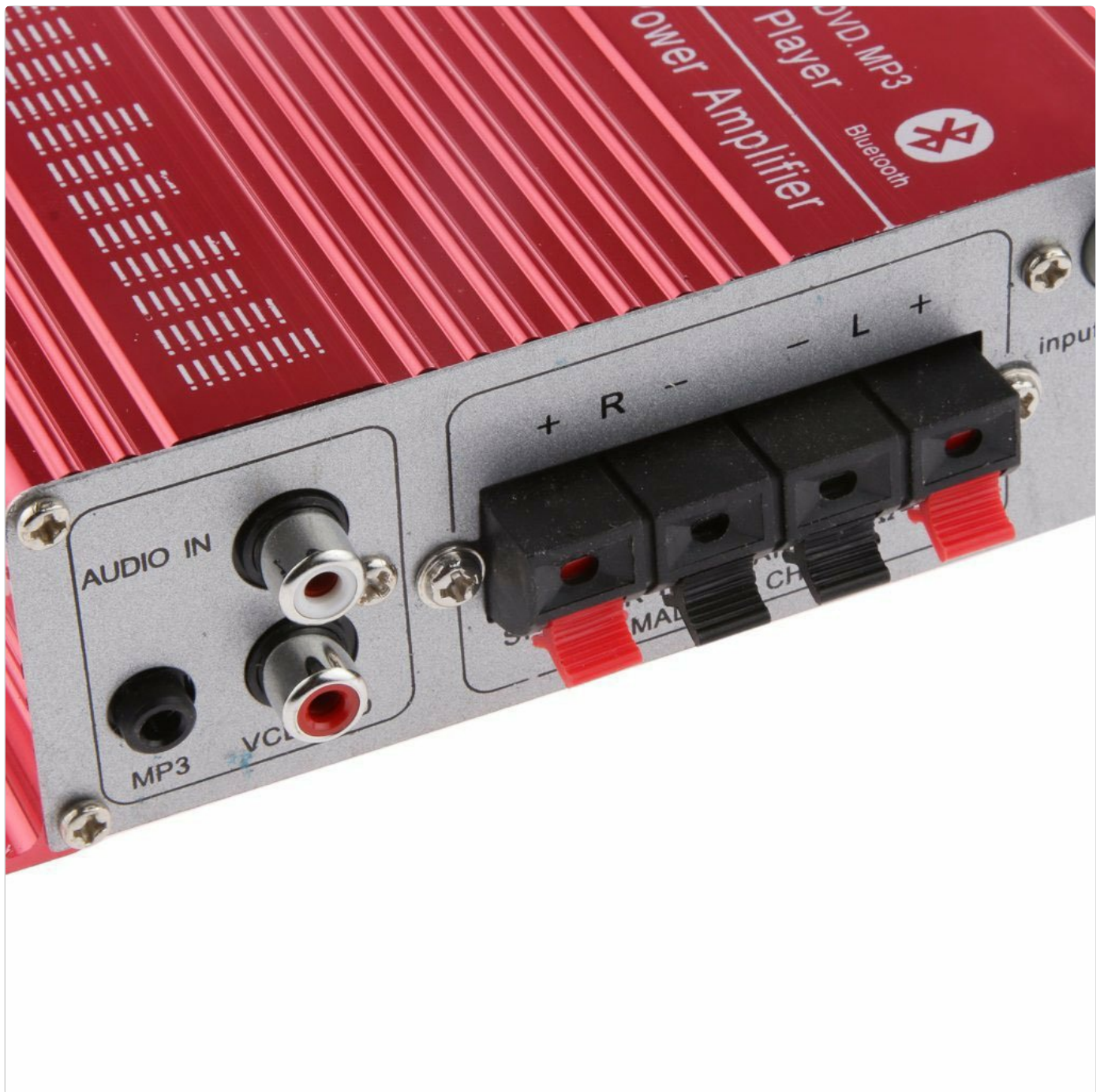
Image 3: Close-up view of the amplifier's rear panel connections. This image shows the Audio In (RCA) ports, Speaker Output terminals (L+/L-, R+/R-), 12V DC power input, and the antenna connection.
