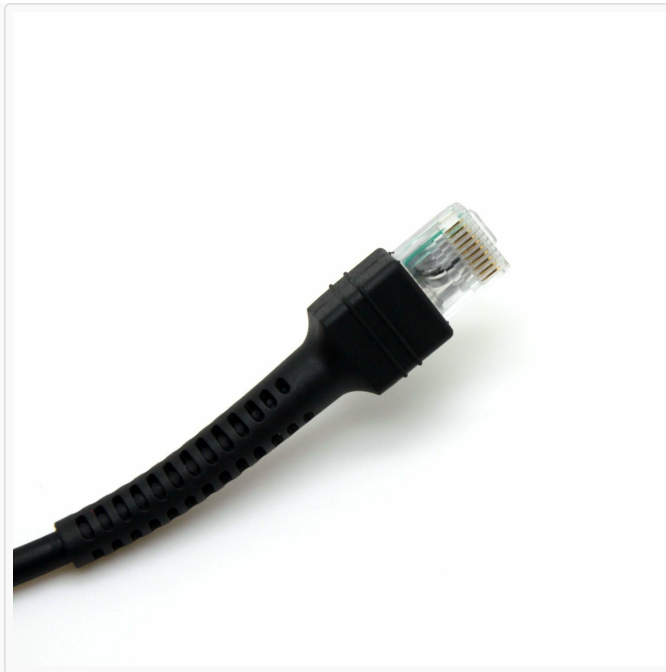
Figure 2: A close-up view of the RJ45 connector, which connects to the Motorola radio's programming port.
