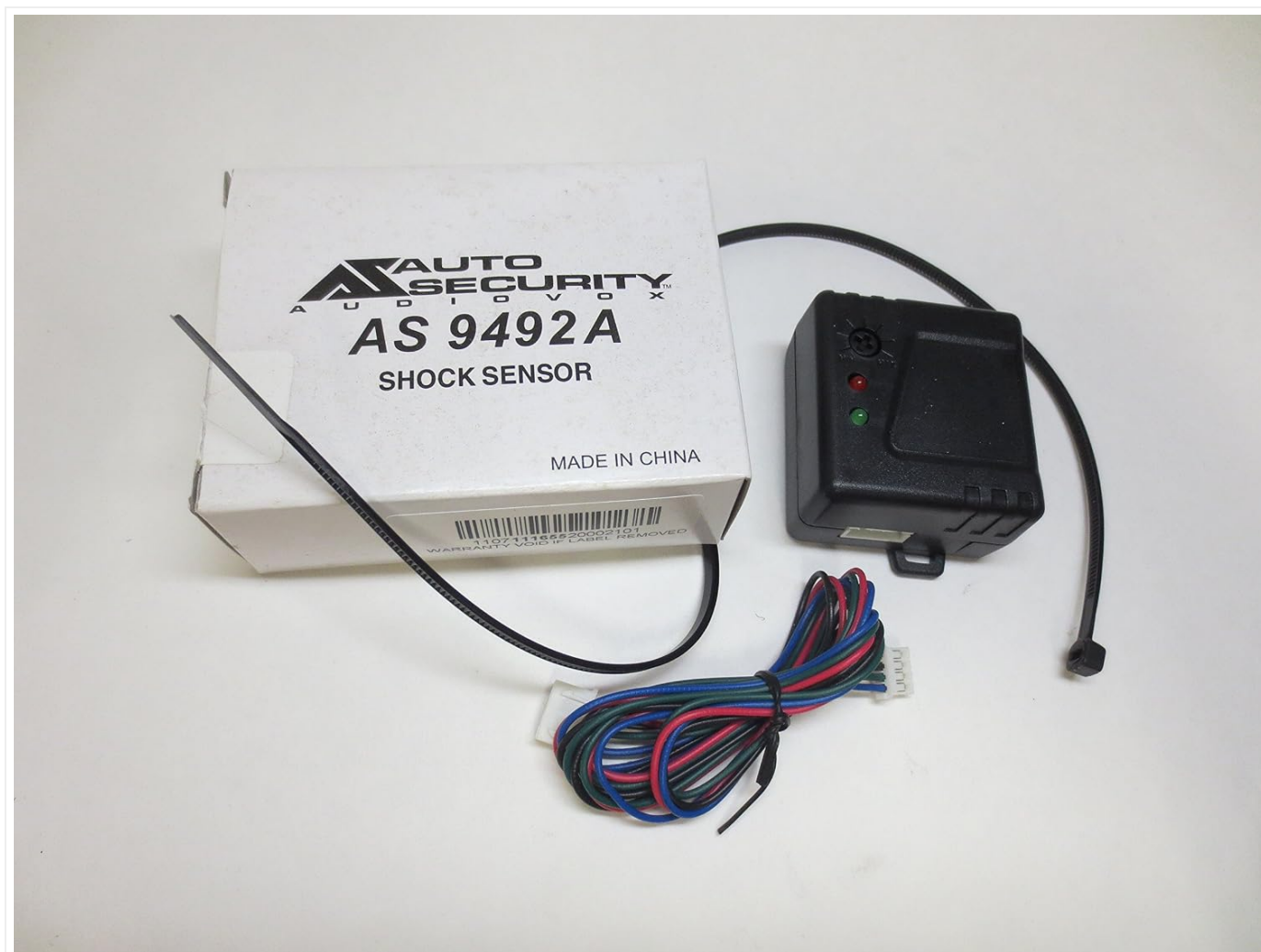
Figure 1: Prestige AS9492a Dual Zone Shock Sensor. The image displays the sensor unit, its packaging box labeled "AUTO SECURITY AUDIOVOX AS 9492A SHOCK SENSOR", and the accompanying wiring harness. The sensor unit itself is a black rectangular device with indicator LEDs (red and green) and a sensitivity adjustment screw.
