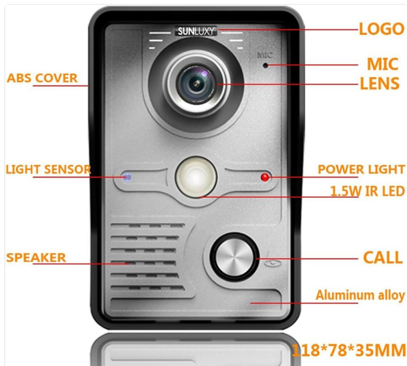
Image 4.1.2: Outdoor Camera Unit Components.
