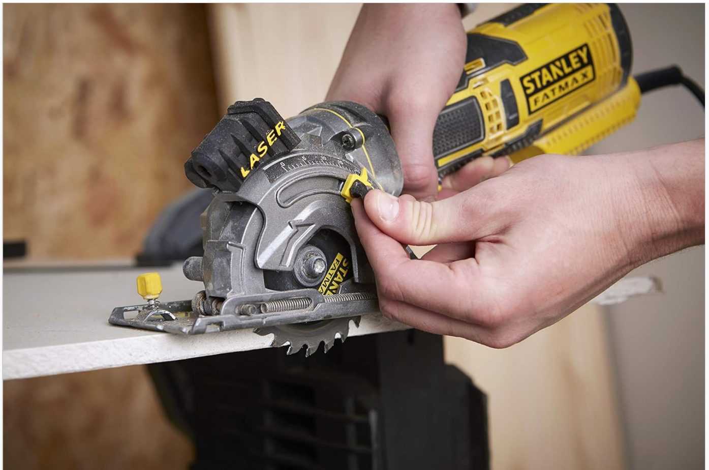
Figure 3.2: Adjusting the cutting depth by manipulating the base plate and securing the lever.
