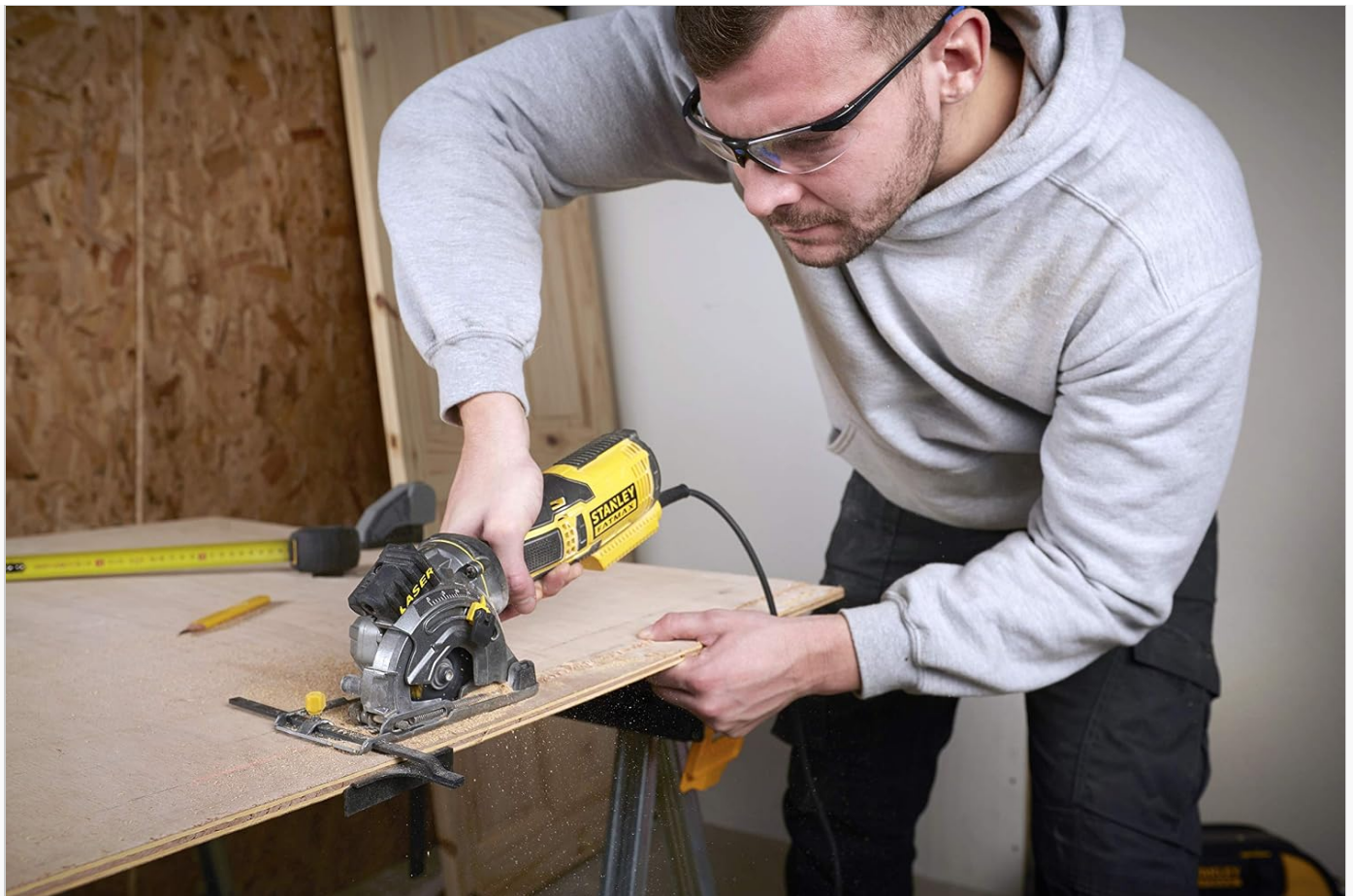
Figure 4.6: The laser guide mechanism on the mini circular saw, designed for enhanced cutting precision.
