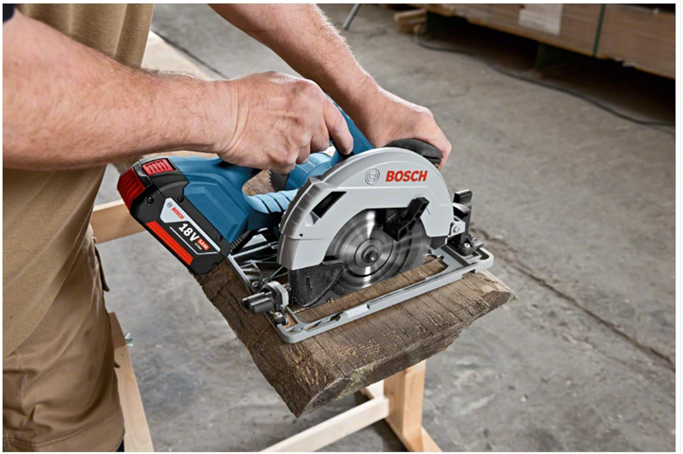
Figure 5.2: Demonstrating the saw's capability to cut through thicker wood sections.
