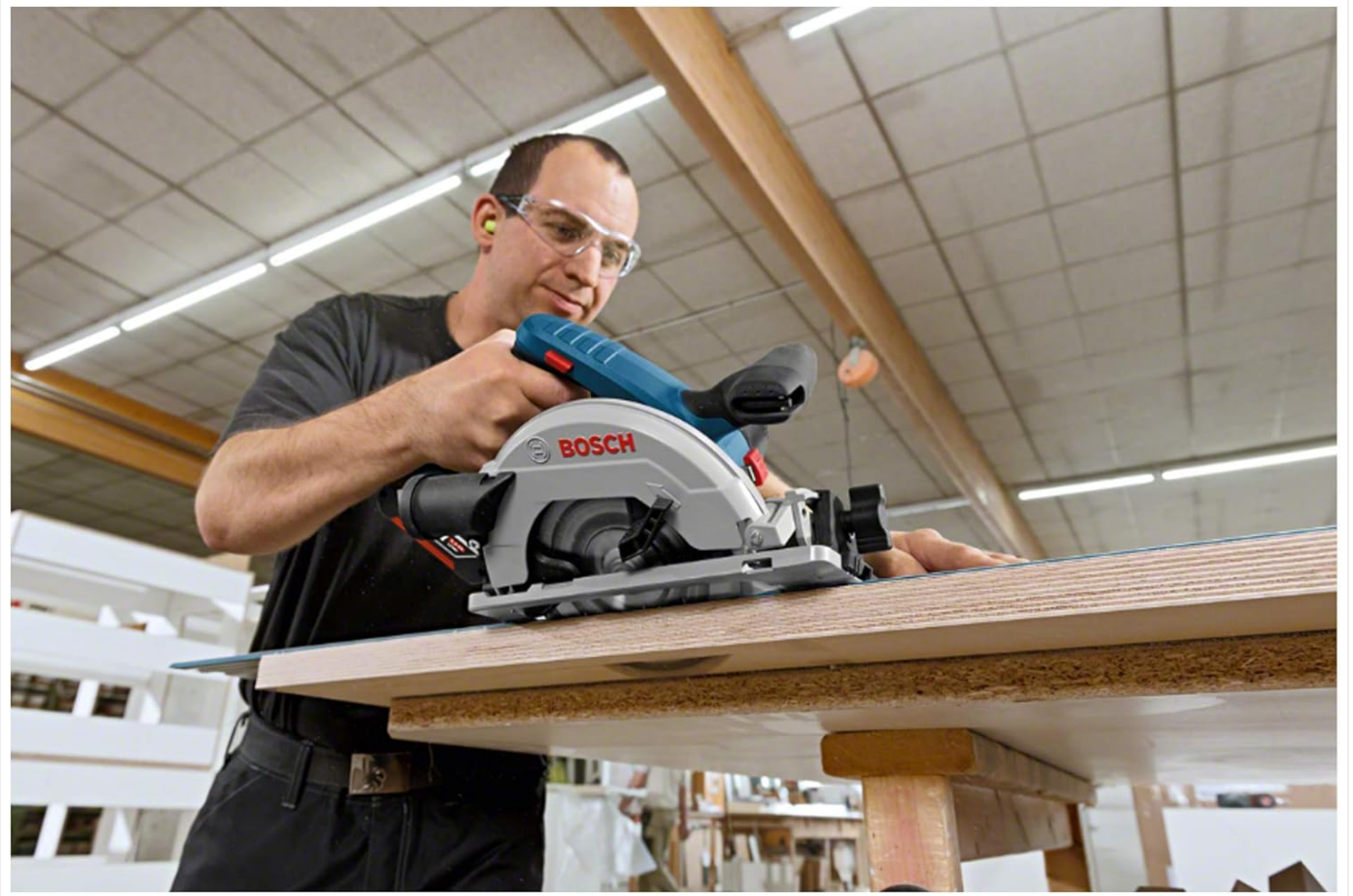
Figure 5.1: Proper technique for cutting a large wooden panel with the circular saw.
