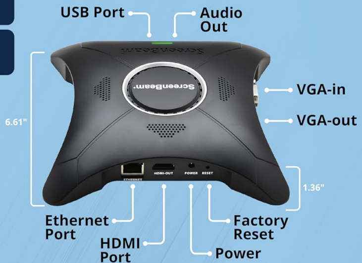
Image 2.1: Visual representation of the ScreenBeam 960 package contents, including the receiver, power supply, HDMI cable, and documentation. Below it, a detailed diagram highlights the device's ports: USB Port, Audio Out, VGA-in, VGA-out, Ethernet Port, HDMI Port, Power, and Factory Reset button.
