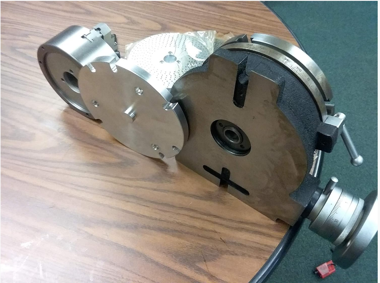
Figure 3.2.5: Disassembled view showing the rotary table, the 3-jaw chuck, and the two index plates with their accessories.
