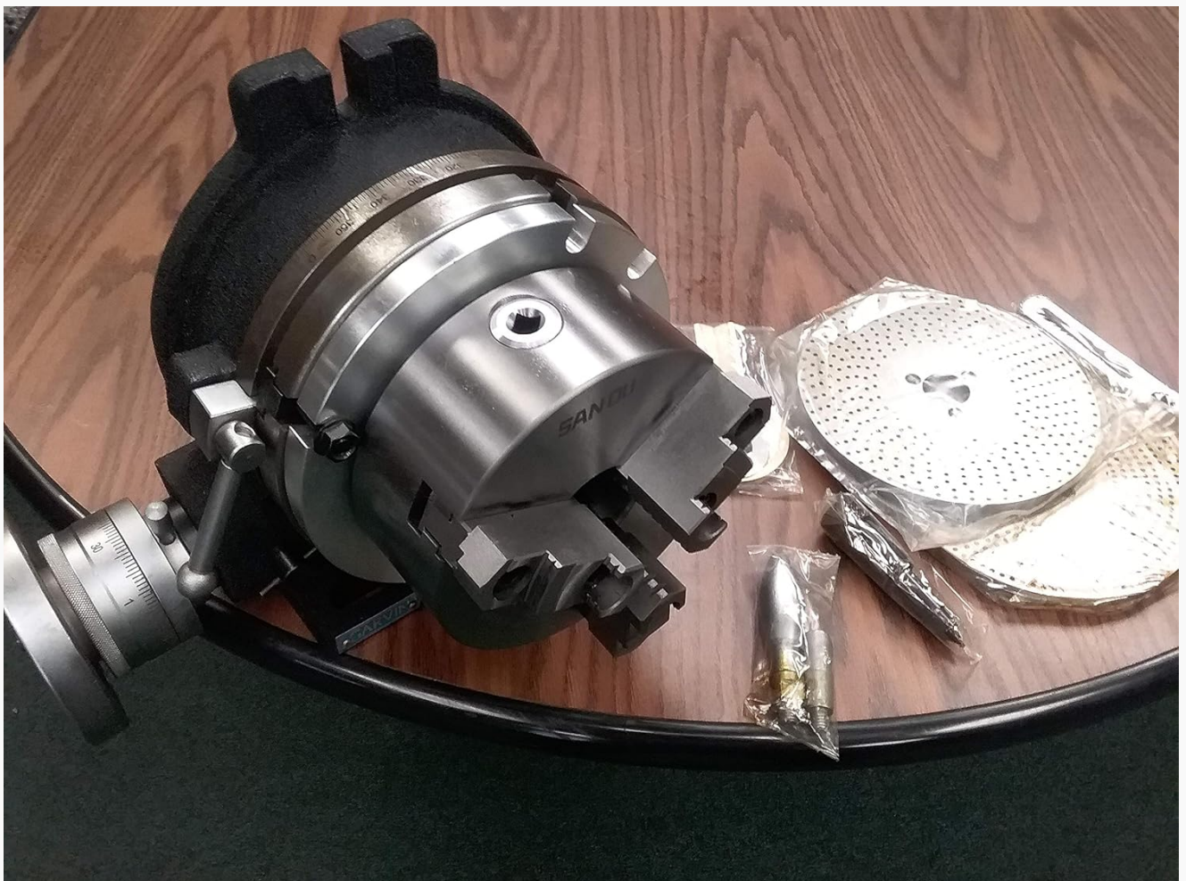
Figure 3.2.1: Overall view of the 8-inch Precision Rotary Table, including the mounted 3-jaw chuck and the two index plates.
