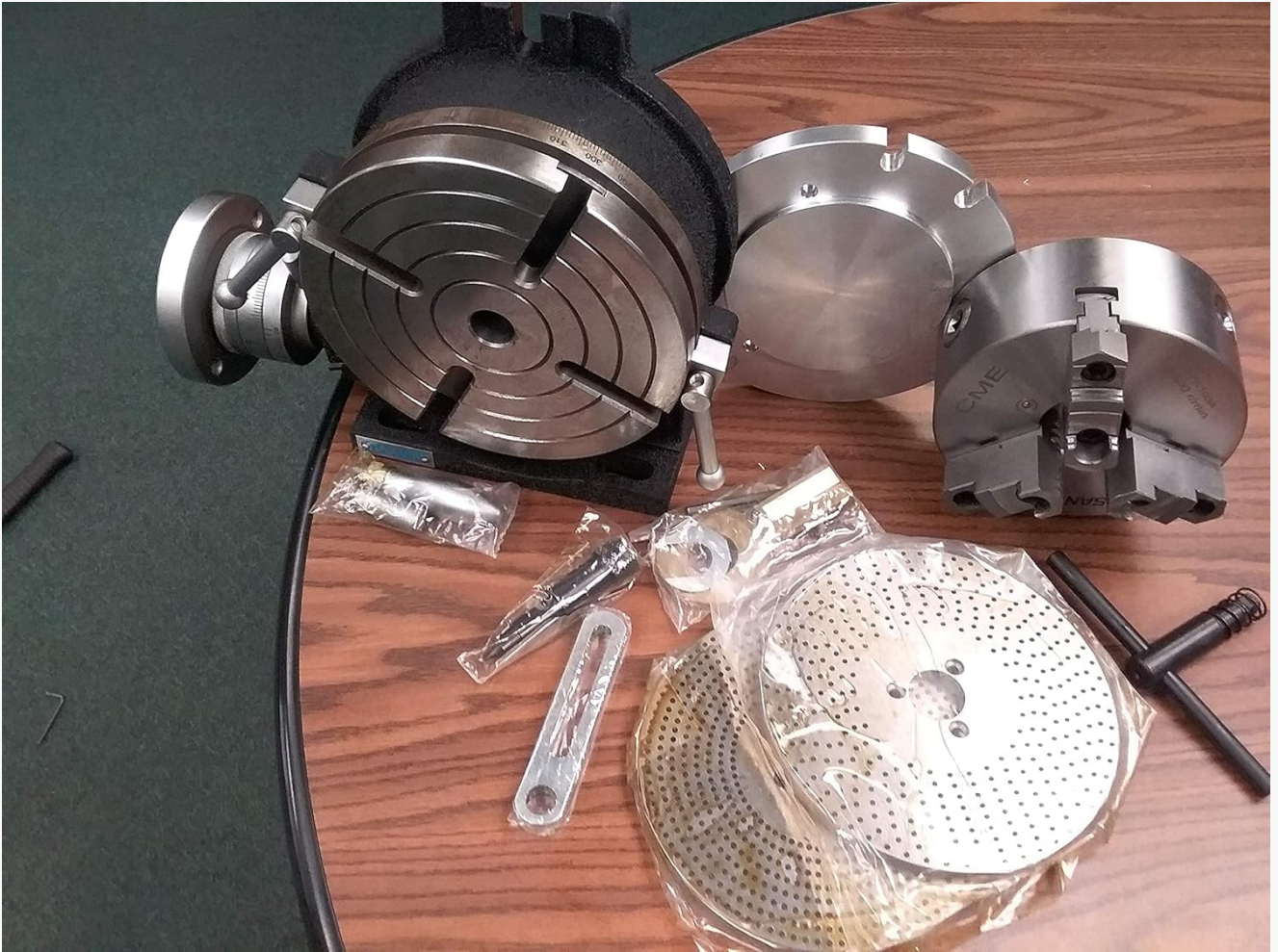
Figure 3.2.5: Disassembled view showing the rotary table, the 3-jaw chuck, and the two index plates with their accessories.
