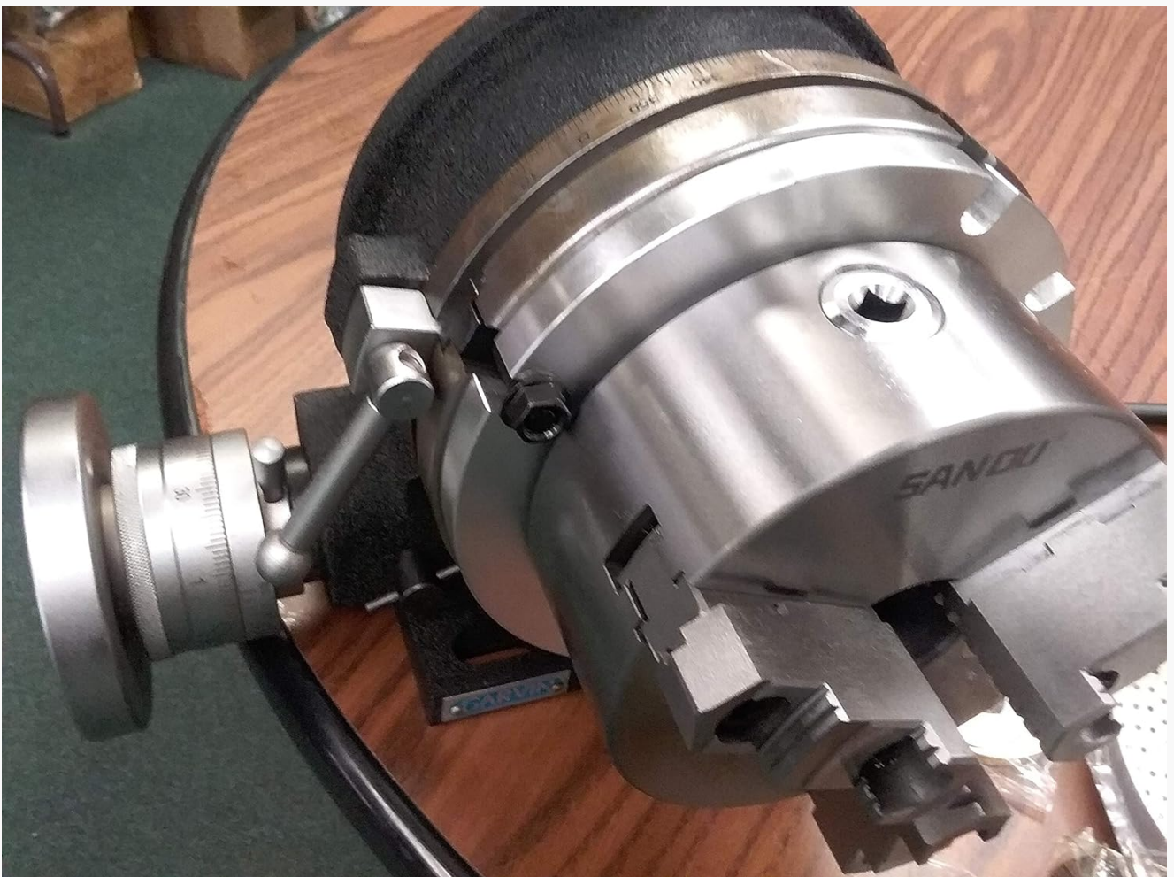
Figure 3.2.2: Top view of the rotary table with the 3-jaw chuck securely mounted, showing the handwheel and locking levers.
