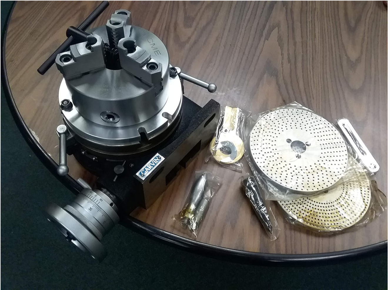
Figure 3.2.2: Top view of the rotary table with the 3-jaw chuck securely mounted, showing the handwheel and locking levers.
