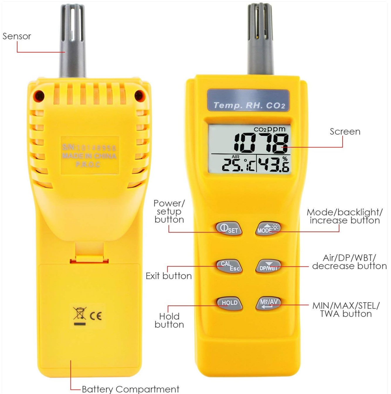
Image: A detailed diagram of the TEKCOPLUS CO2 Detector, showing the location and function of its various parts, including the sensor, LCD screen, power/setup button, mode/backlight button, calibration/exit button, DP/WBT/decrease button, hold button, MIN/MAX/STEL/TWA button, and battery compartment.
