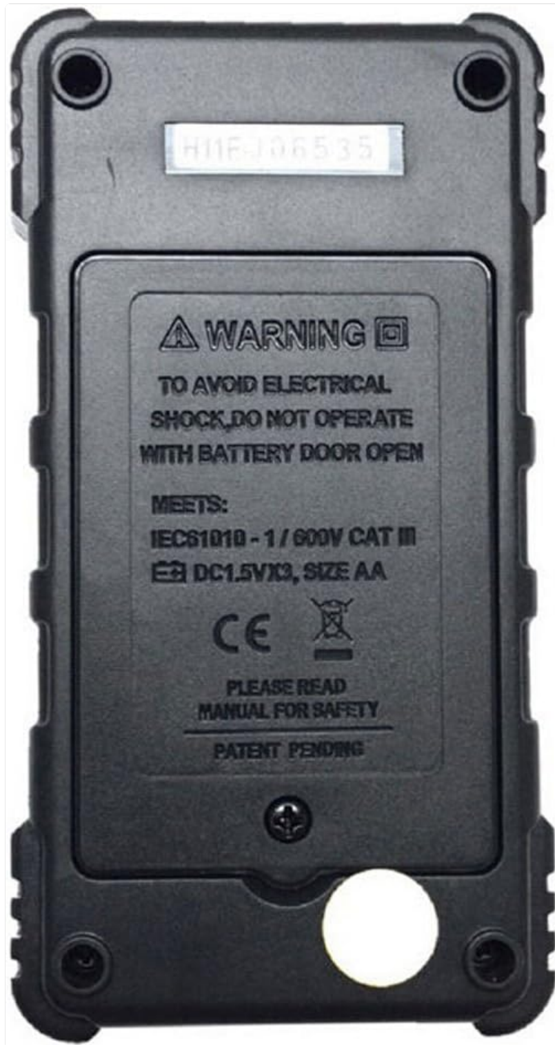
Figure 2.1: Rear view of the MS5900, highlighting the battery compartment and the warning against operation with the battery door open to prevent electrical shock.
