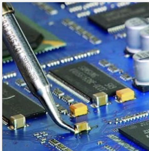
Figure 5.5: Illustrates the proper technique for soldering a surface-mount component onto a printed circuit board.
