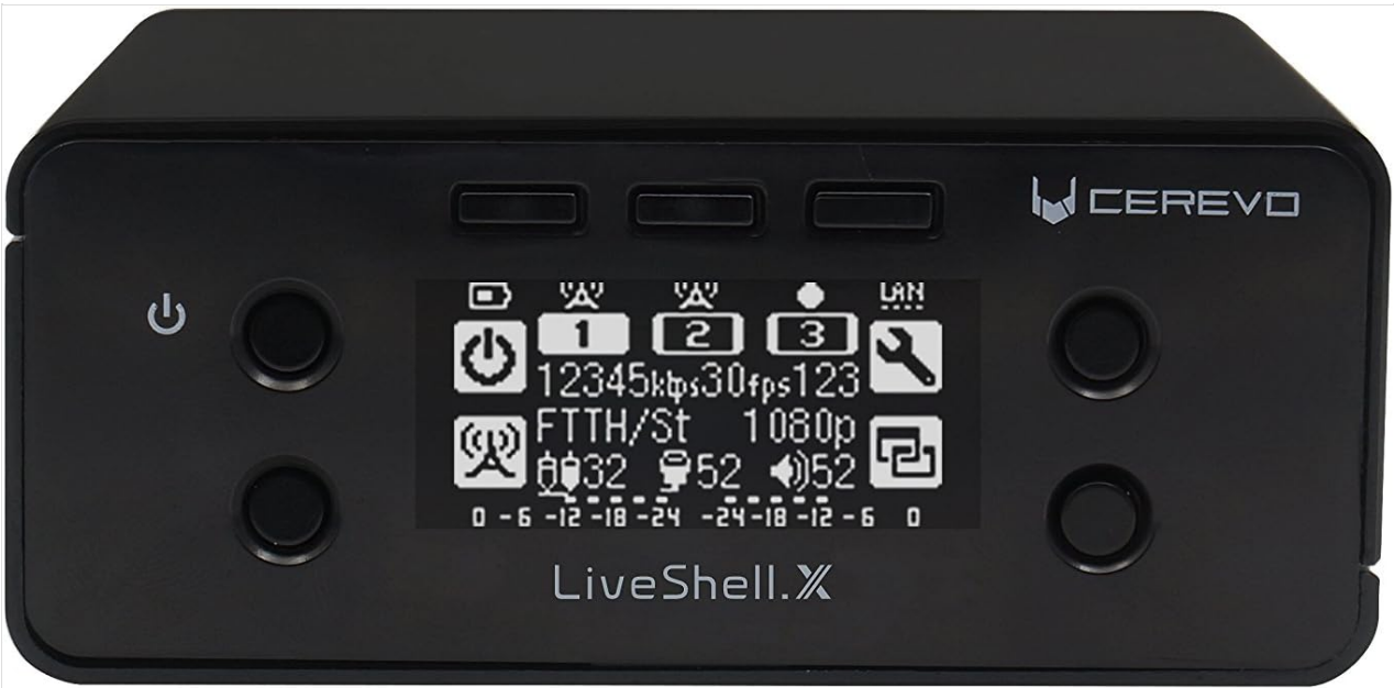
Figure 2.1: Front view of the Cerevo LiveShell X with its OLED display.
