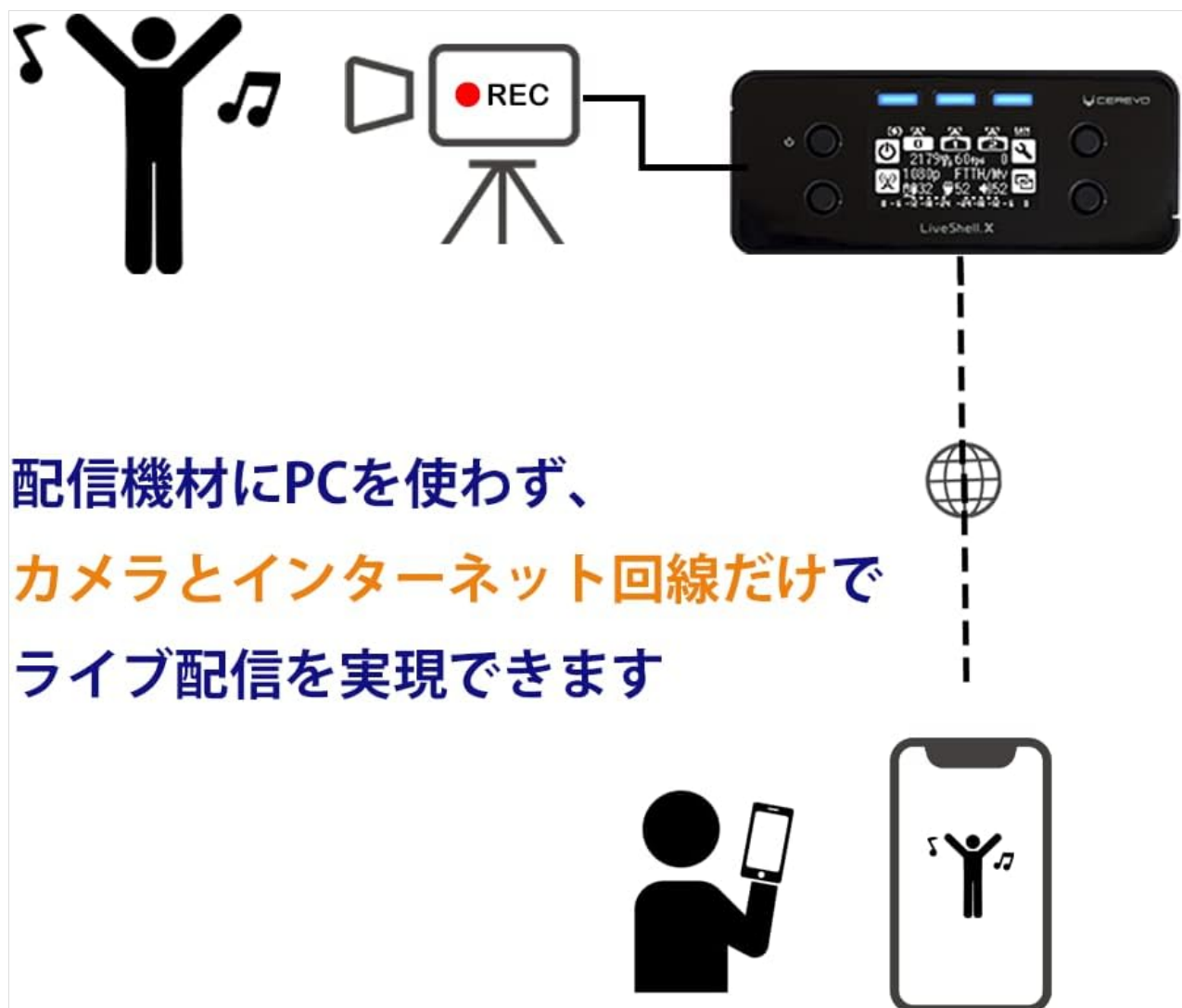
Figure 3.1: PC-less live streaming setup with LiveShell X.
