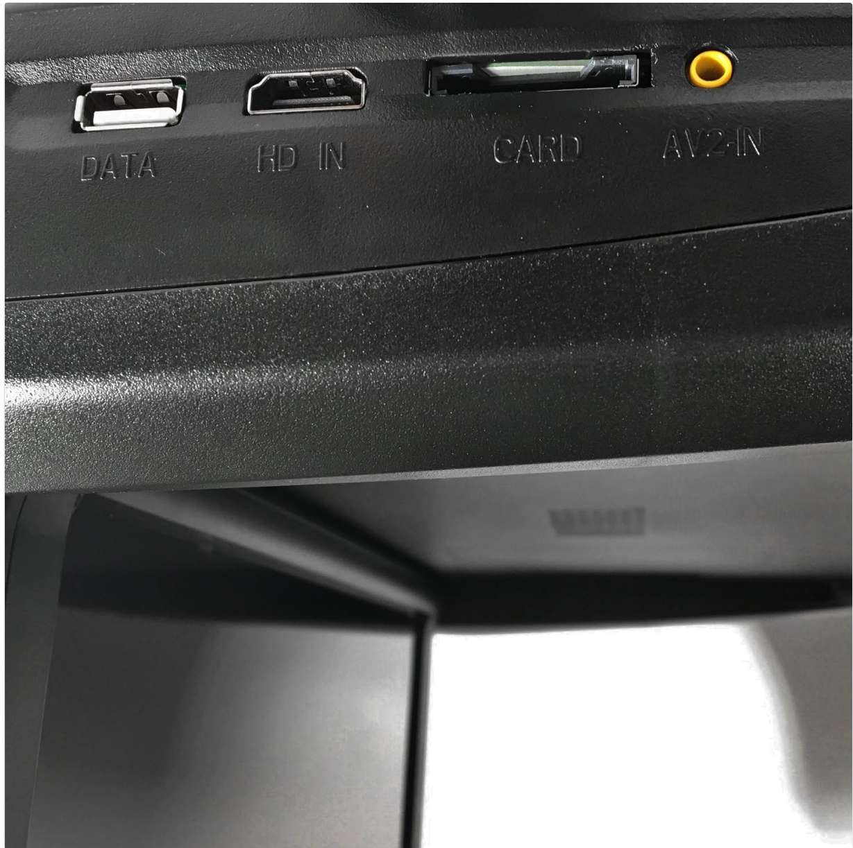
Image: Close-up view of the input/output ports on the side of the monitor, labeled "DATA" (USB), "HD IN" (HDMI), "CARD" (SD), and "AV-IN".
