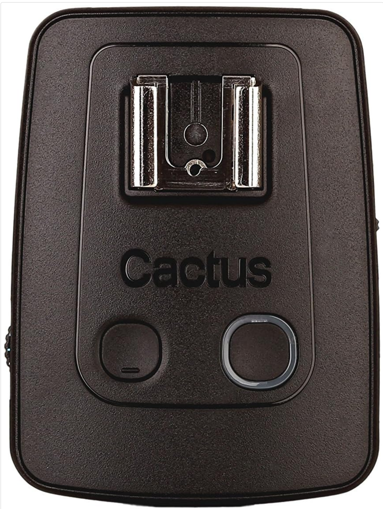
Figure 3.2: Top-down view of the Cactus V6IIIS. This perspective clearly shows the hot shoe connection point and the two prominent control buttons on the device's surface.
