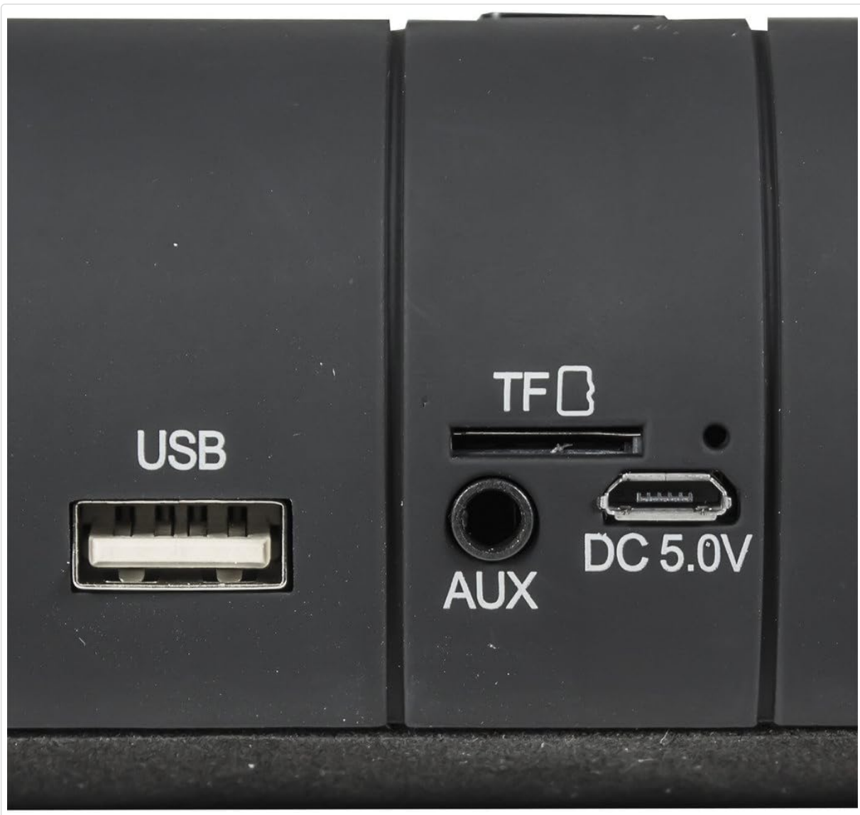
Close-up of the input ports on the Billboard BB783 speaker, including USB, AUX, TF (Micro SD) card slot, and DC 5.0V charging port.
