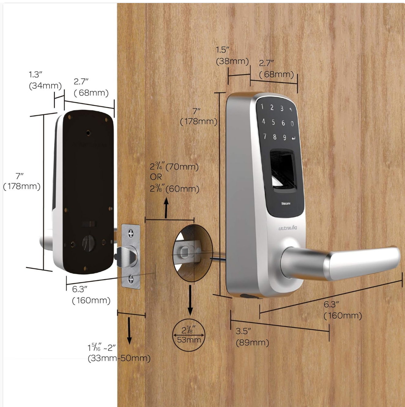
Image: Technical drawing illustrating the dimensions of the ULTRALOCK UL3 BT Smart Lock and the required door preparation measurements for installation, including door thickness, backset, and bore hole sizes.
