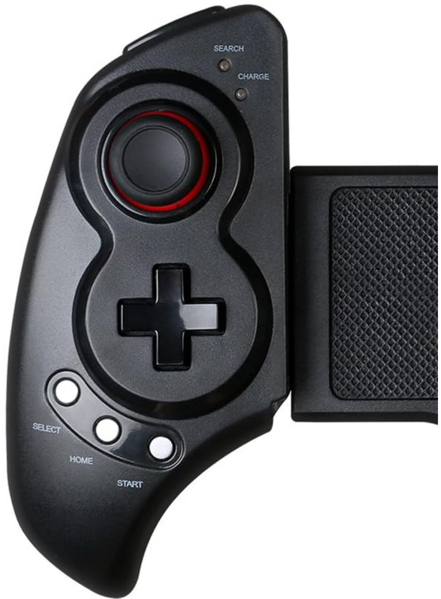
Figure 2: Left side of the controller, featuring the D-pad and left analog stick, designed for a natural feel with arc-shaped buttons.
