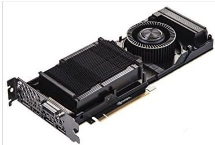
Figure 2: Rear view of the NVIDIA GTX TITAN X, highlighting the available display output ports.
