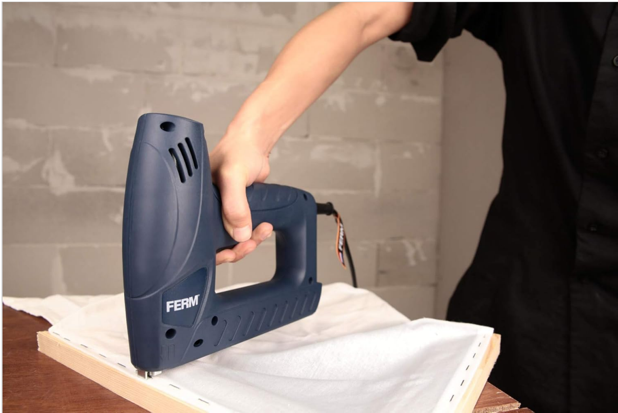
Figure 5: Proper handling and use of the tacker on a workpiece.
