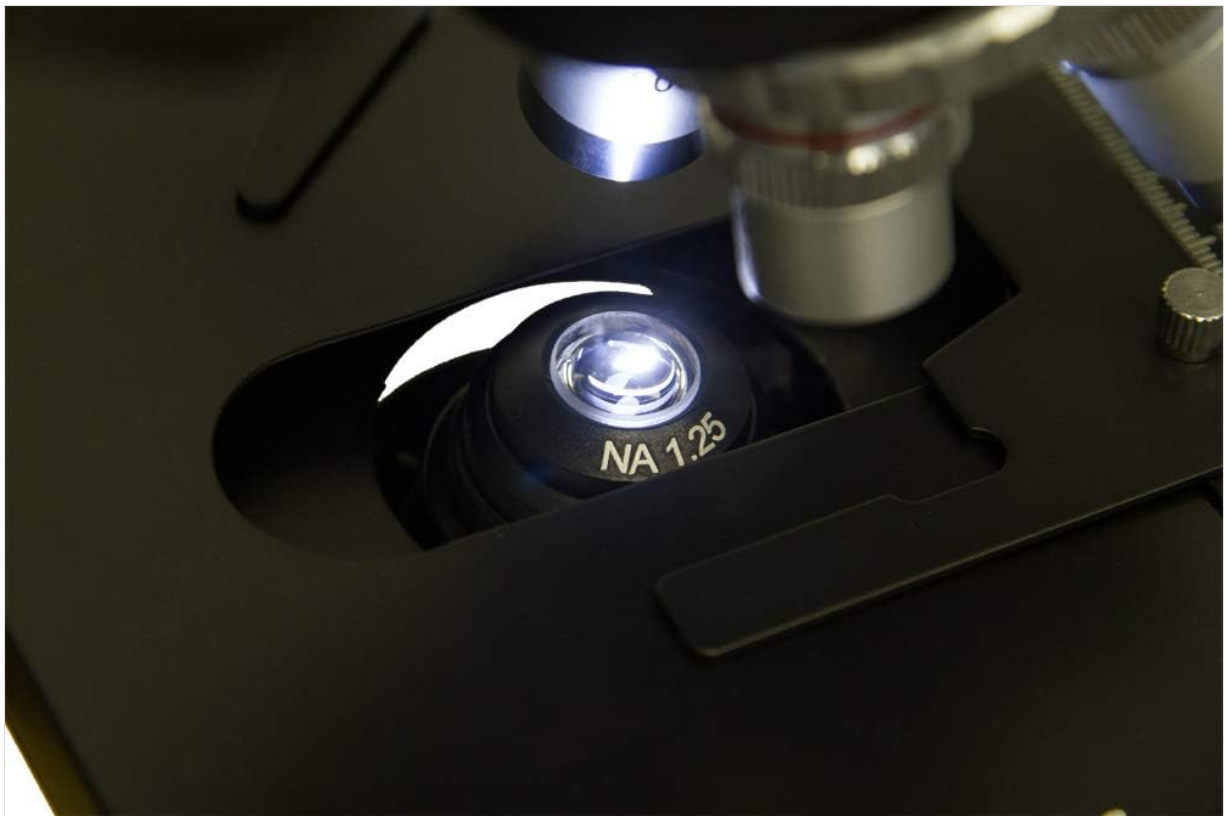
Figure 4.2: View of the illuminated condenser and objective lens from below the stage.
