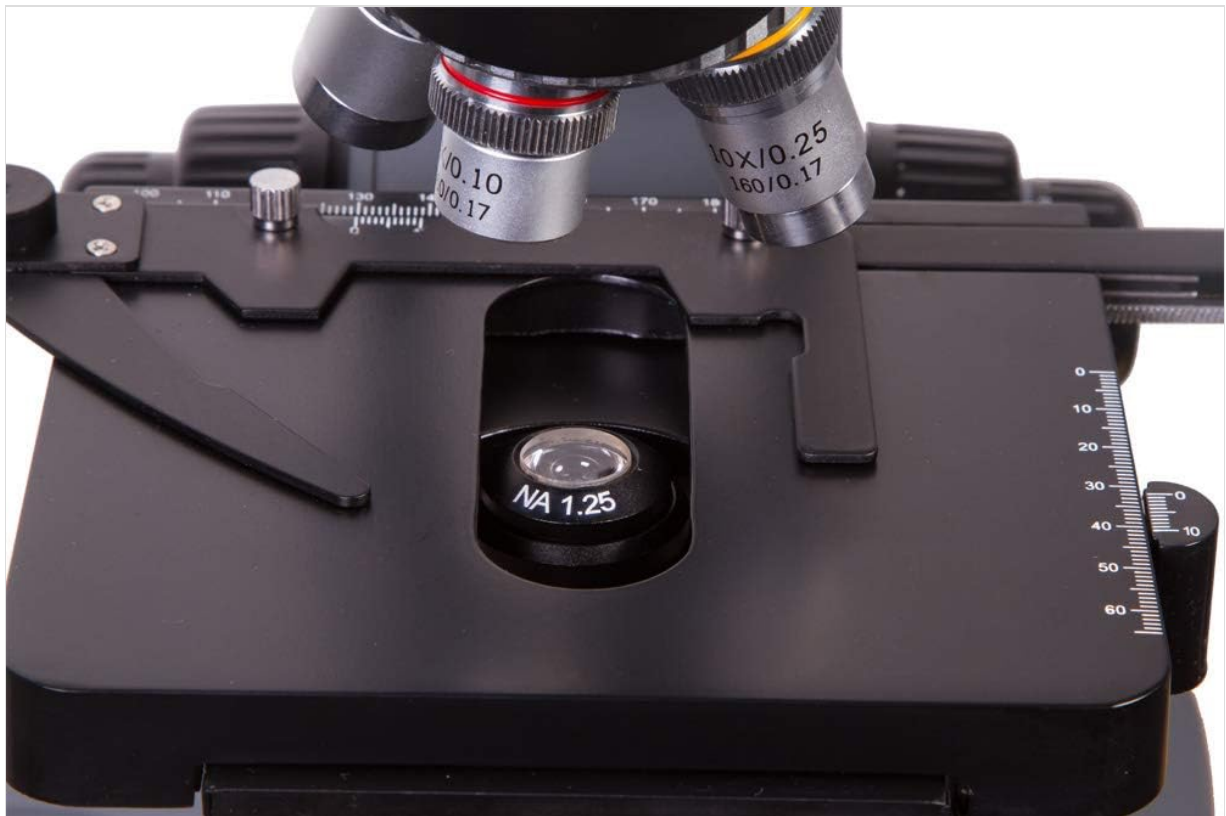
Figure 4.1: Close-up view of the mechanical stage with the condenser and iris diaphragm visible below.
