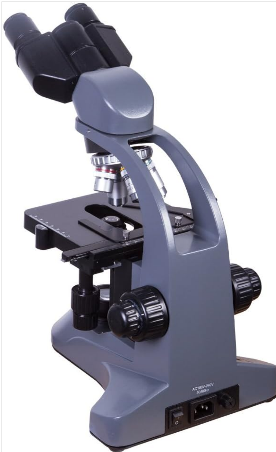
Figure 3.1: Rear view of the microscope showing the power input and switch.
