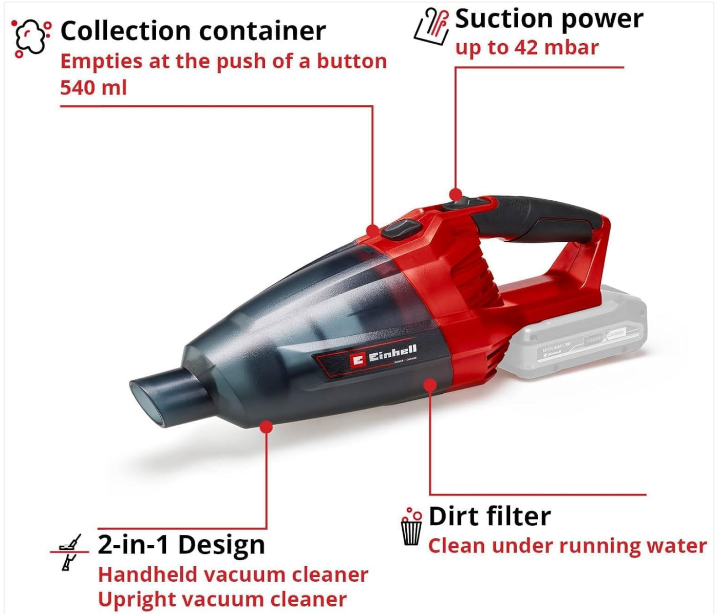
Figure 3.2: Key features of the vacuum cleaner, highlighting the collection container (540 ml), suction power (up to 42 mbar), 2-in-1 design (handheld/upright), and washable dirt filter.
