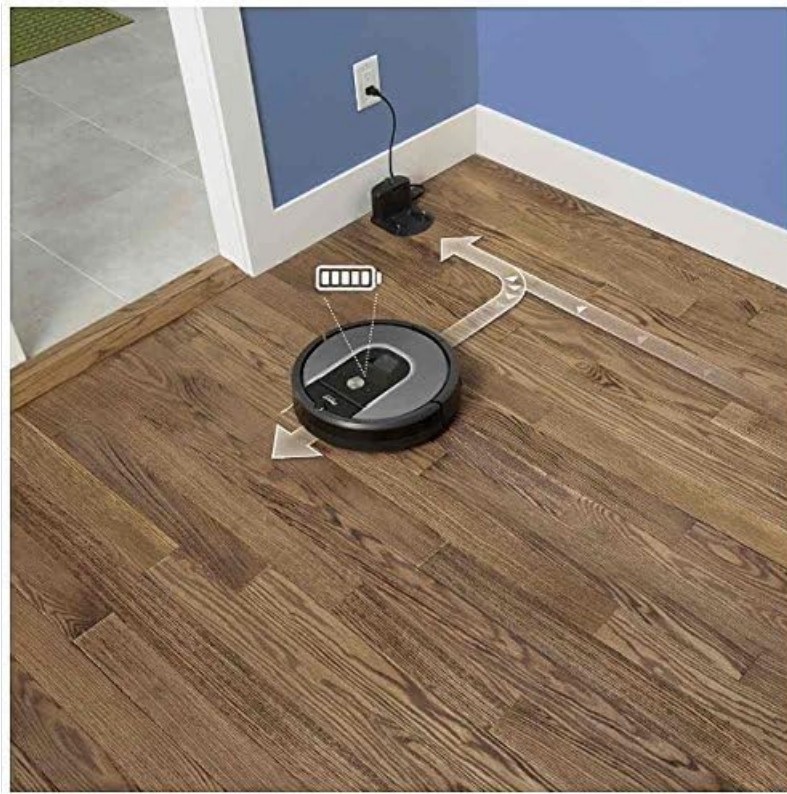
Figure 2: The Roomba 960 automatically returns to its Home Base for charging.
