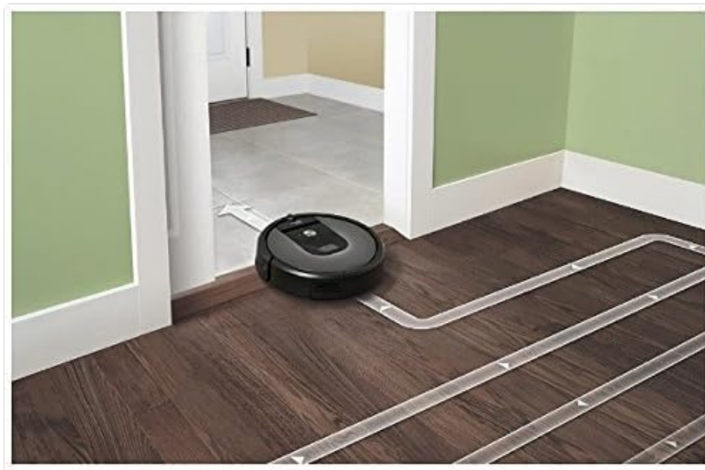
Figure 4: The Roomba 960 navigating around a Virtual Wall barrier.
