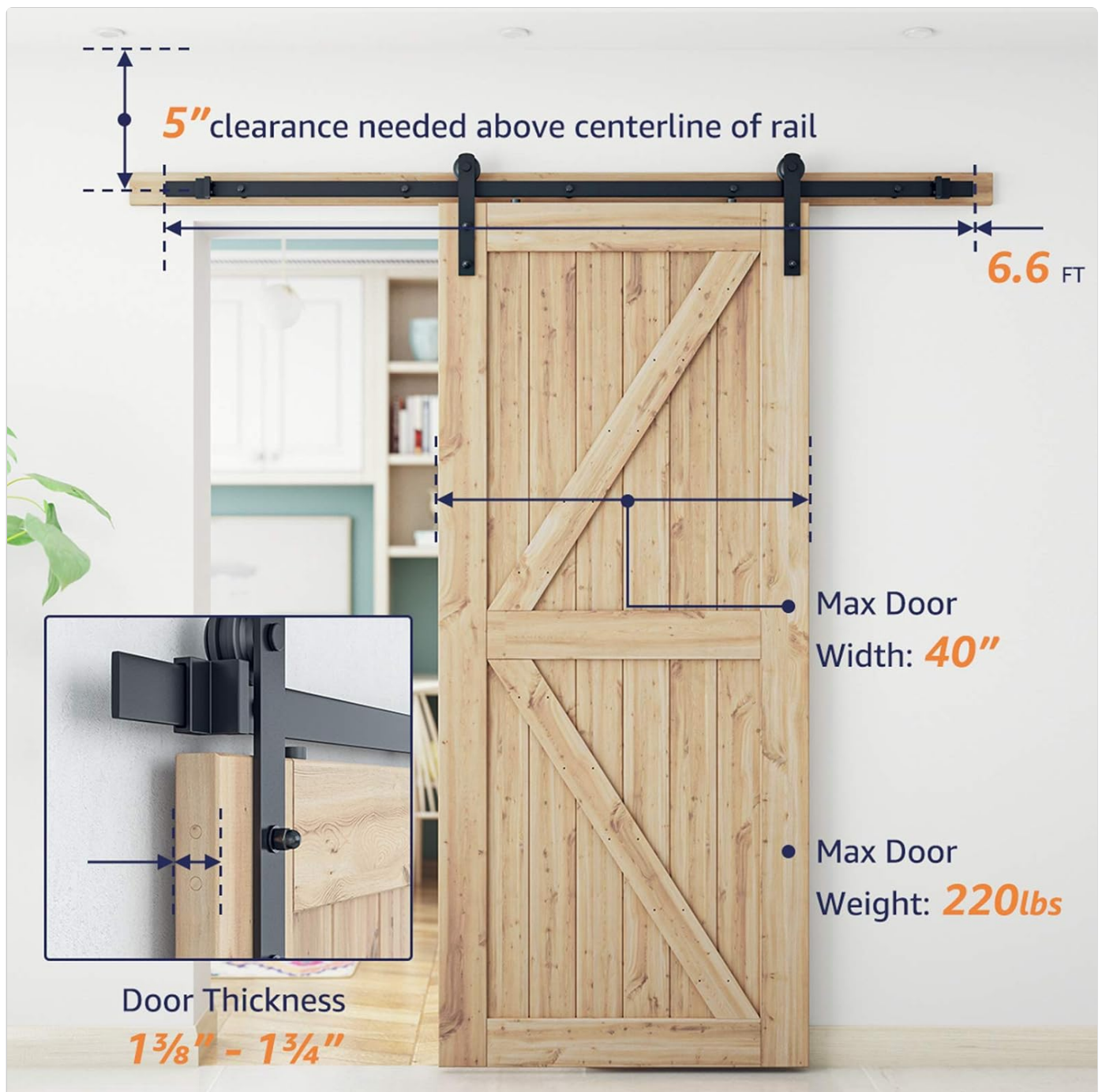
Key dimensions and maximum door specifications for installation.
