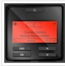
Figure 5.1: This image displays the LCD screen showing a 'Connect Battery' alarm, indicating that the internal battery is not properly connected or detected, and backup power is unavailable.
