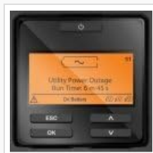
Figure 3.2: The LCD display indicating a 'Utility Power Outage' and the remaining battery run time, demonstrating the UPS's response to power interruptions.
