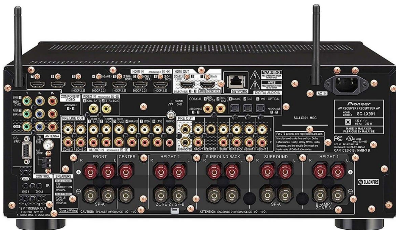
Image 1: Rear panel view of the Pioneer Elite SC-LX901 AV Receiver. This image displays all available input and output connections, including HDMI, analog audio, digital audio, speaker terminals, network port, and antenna connections. Key sections are labeled for easy identification of connection points for various home theater components.
