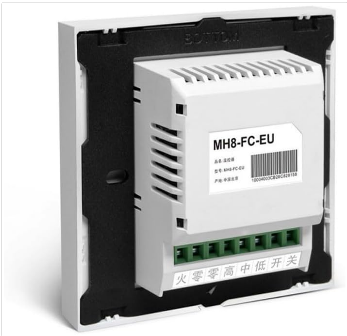
Figure 4.2: Rear view of the MCO Home MH8-FC4 Thermostat. This image displays the terminal block for electrical connections and the product label indicating the model MH8-FC-EU.
