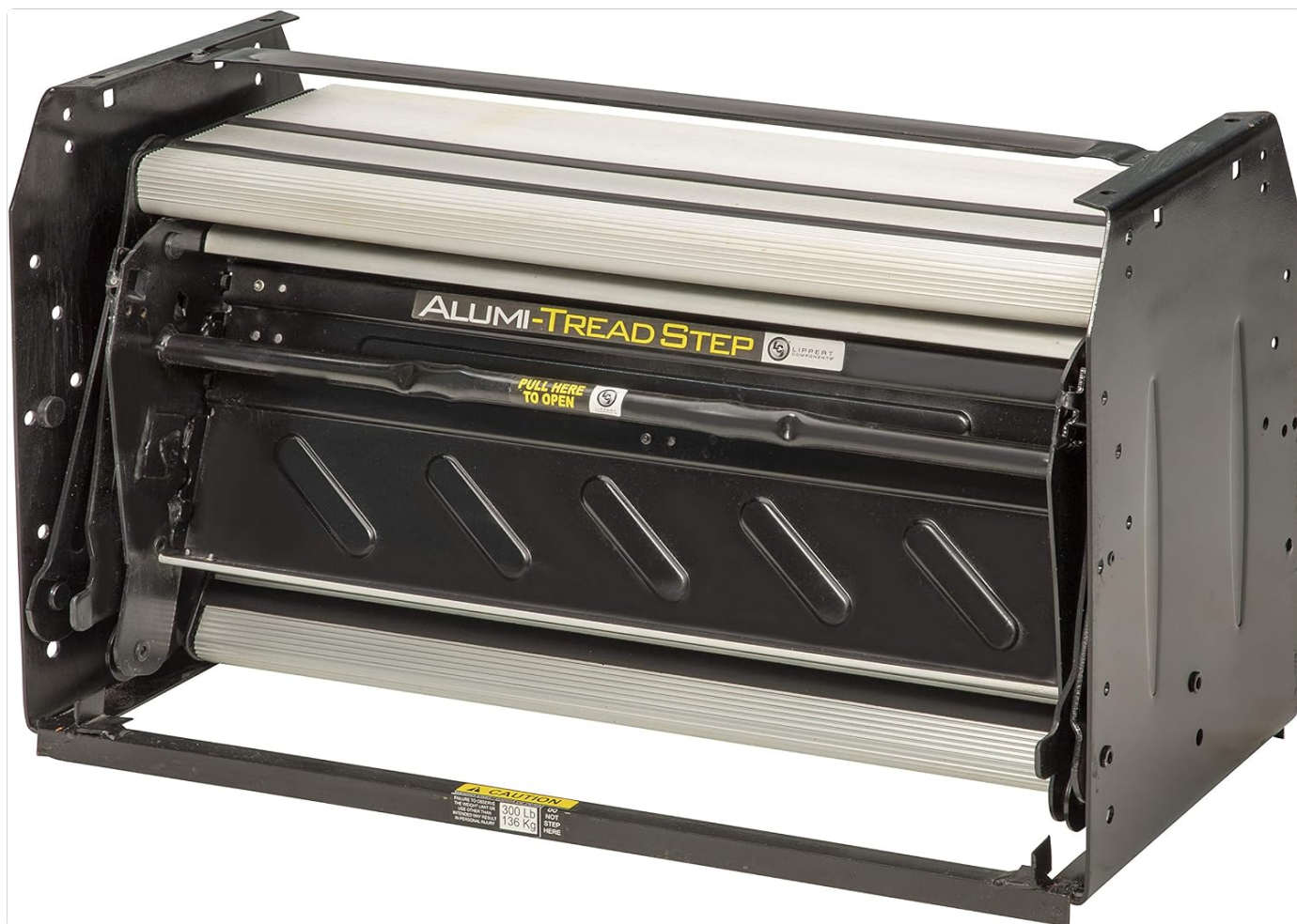
Figure 3.2: Front view of the Alumi-Tread Triple Manual Step in its folded, stored position.
