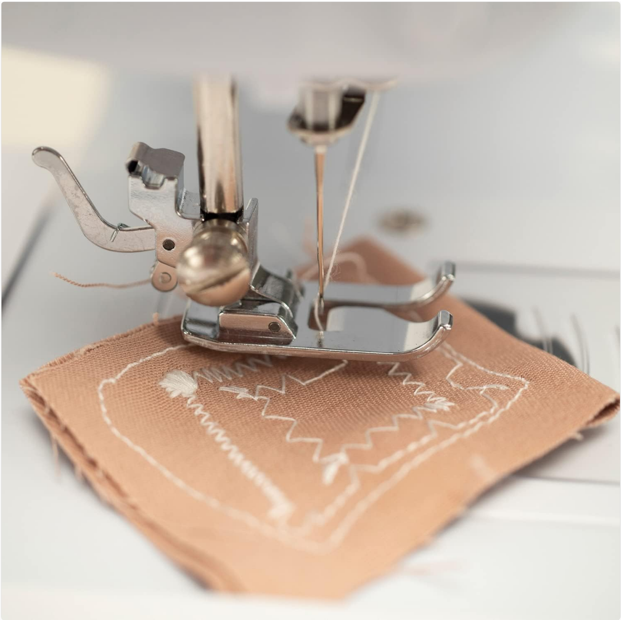
Figure 4: Close-up of the needle and presser foot in action.
