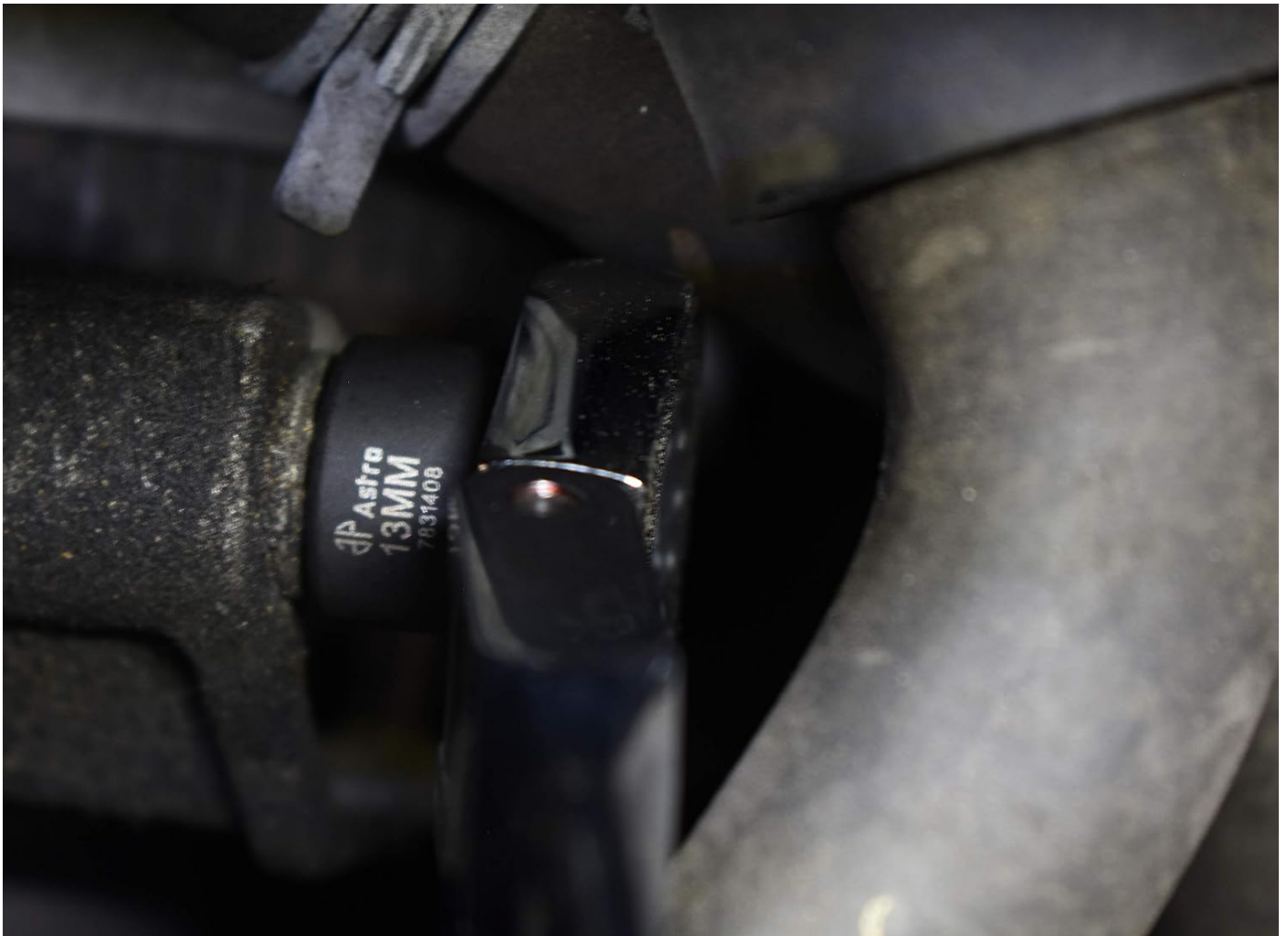
Figure 3: Demonstrating the low-profile access in a confined space.
